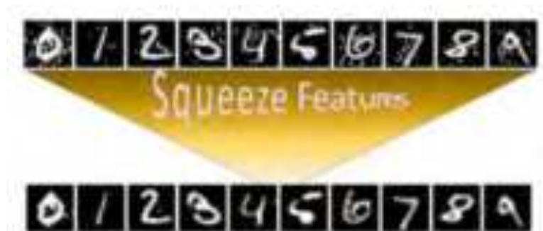
Figure 4. An example of Feature Squeezing, which smooths inputs to remove adversarial inputs [
